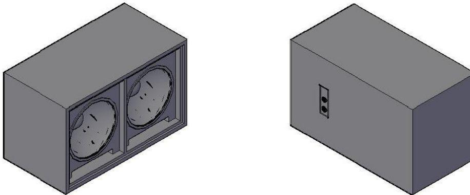
Being a subwoofer studio monitor, it performs well with SM1 Loudspeaker. for an optimal performance, use one SUBSM1 each two SM1. Place the sub in the middle of the two satellites trying to keep aligned the emission source of all speakers.
